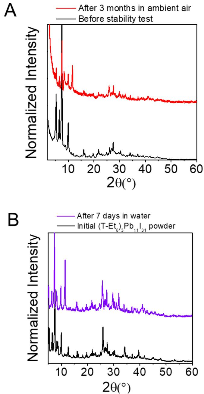
**Figure 4.** (A) PXRD pattern of (T-Et<sub>6</sub>)<sub>3</sub>Pb<sub>11</sub>I<sub>31</sub> crystals before and after 3 months stored in ambient air. (B) PXRD pattern of (T-Et<sub>6</sub>)<sub>3</sub>Pb<sub>11</sub>I<sub>31</sub> crystals before and after 7 days in water.
