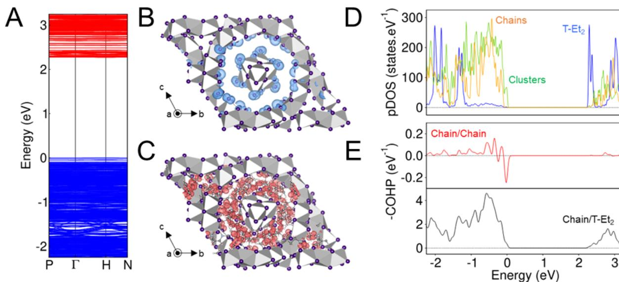
**Figure 9.** (A) DFT computed band structures of (T-Et<sub>6</sub>)<sub>3</sub>Pb<sub>11</sub>I<sub>31</sub>. (B) and (C) Partial charge densities taken at the valence band maximum (VBM, blue) and the conduction band minimum (CBM, red), respectively. For clarity, T-Et<sub>6</sub> cations are not depicted for the VBM that is distributed over [Pb<sub>11</sub>I<sub>31</sub>]<sup>9-</sup> chains, while the CBM is composed by contributions of the T-Et<sub>6</sub> cations. Identical
