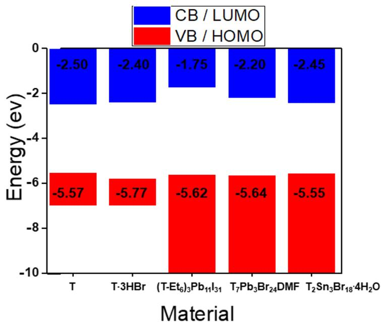
**Figure 8.** Band alignment diagram with valence band maximum energies determined from Photoemission Yield Spectroscopy in Air (PYSA) measurements of T, T·3HBr, 3D (T-Et<sub>6</sub>)<sub>3</sub>Pb<sub>11</sub>I<sub>31</sub>, 0D T<sub>7</sub>Pb<sub>3</sub>Br<sub>27</sub>·DMF and 0D T<sub>2</sub>Sn<sub>3</sub>Br<sub>18</sub>·4H<sub>2</sub>O·0.5Br<sub>2</sub>.
