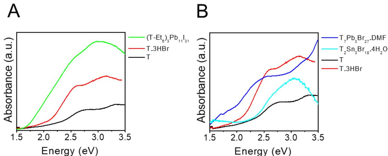
**Figure 5.** Solid-state optical absorption spectra of compounds (A)  $(\text{T-Et}_6)_3\text{Pb}_{11}\text{I}_{31}$  alongside T and T.3HBr, (B)  $\text{T}_7\text{Pb}_3\text{Br}_{27}\cdot\text{DMF}$  and  $\text{T}_2\text{Sn}_3\text{Br}_{18}\cdot 4\text{H}_2\text{O}$  alongside T and T.3HBr.
