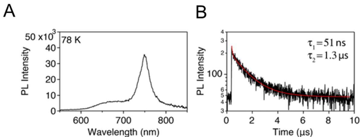
**Figure 6.** Steady-state PL emission spectrum for  $(\text{T-Et}_6)_3\text{Pb}_{11}\text{I}_{31}$  at 78 K (A) followed by the time-resolved PL dynamics at 78 K (B). The compound shows biexponential recovery dynamics with lifetimes of 51 ns and 1.3  $\mu\text{s}$ .
