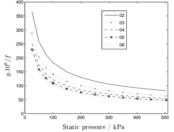
Figure 7. Theoretical half-widths for radial modes from (0,2) to (0,6) as function of the static pressure.
