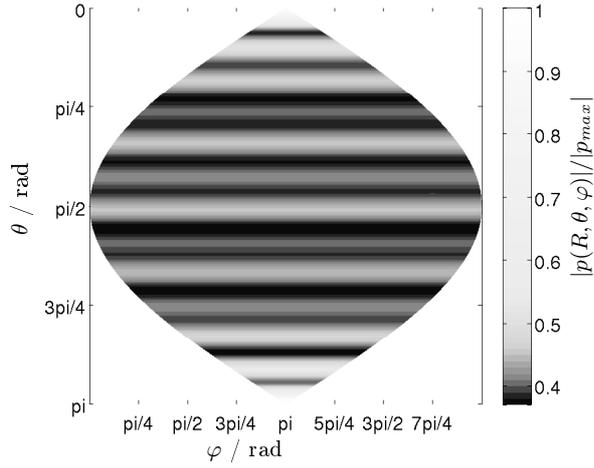
Figure 3. Acoustic pressure on the wall of a spherical cavity at the resonance frequency of the (0,5) radial mode, at the static pressure 25 kPa.
