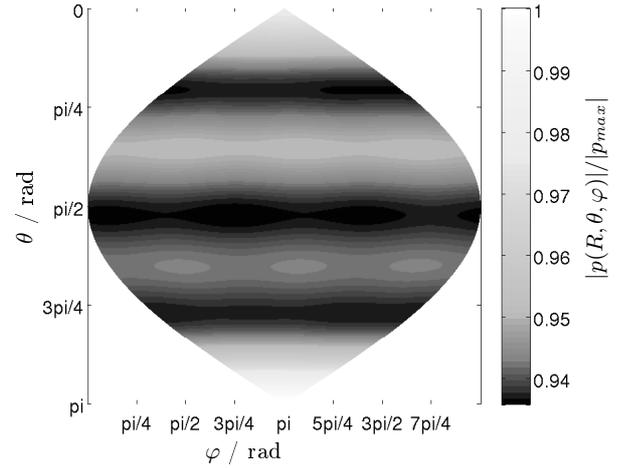
Figure 4. Acoustic pressure on the wall of a spherical cavity at the resonance frequency of the (0,2) radial mode, at the static pressure 500 kPa.
