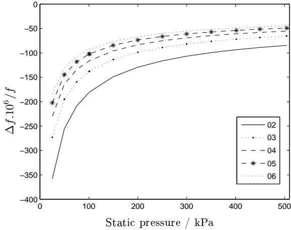
Figure 6. Frequency shifts for radial modes from (0,2) to (0,6) as function of the static pressure.
