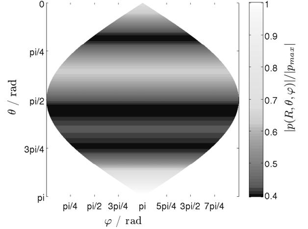
Figure 2. Acoustic pressure on the wall of a spherical cavity at the resonance frequency of the (0,2) radial mode, at the static pressure 25 kPa.
