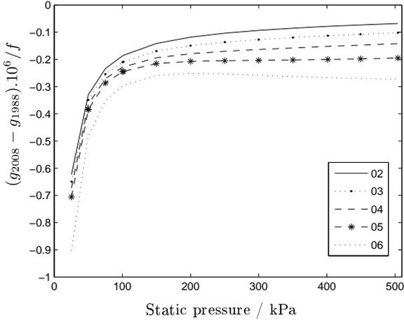
Figure 9. Differences between the half-widths calculated according to actual and previous theories for radial modes from (0,2) to (0,6) as function of the static pressure.
