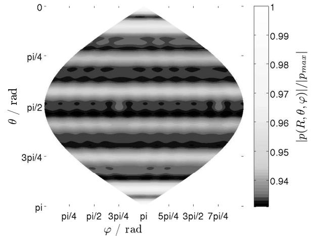
Figure 5. Acoustic pressure on the wall of a spherical cavity at the resonance frequency of the (0,5) radial mode, at the static pressure 500 kPa.
