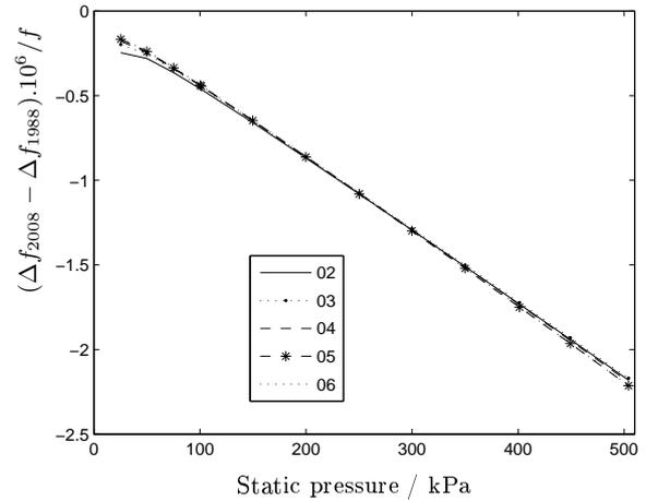
Figure 8. Differences between the frequency shifts calculated according to actual and previous theories for radial modes from (0,2) to (0,6) as function of the static pressure.
