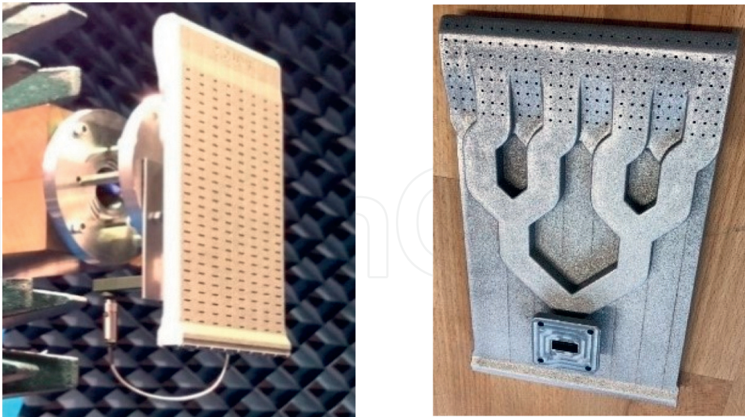
Figure 9. SLM printed compact ridged linearly polarized 2D leaky-wave array with folded beam-forming network.
