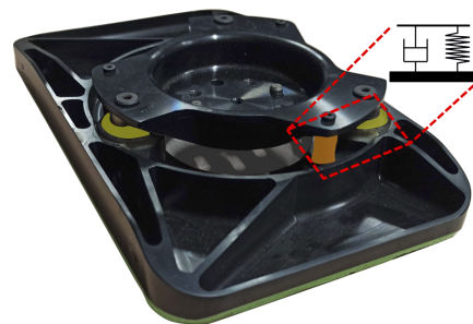
Fig. 19. Rubber bushes (yellow) and dampers (orange) under HRP-4 ankles that induce non-modeled flexibilities.
