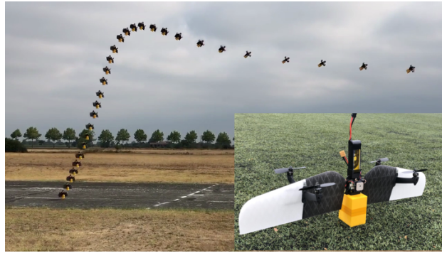
Fig. 2 Baseline vehicle and sequential imagery of vertical take-off and transition in a test flight [27]
