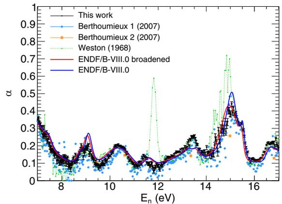
FIG. 12. This work compared to ENDF/B-VIII.0 and the experimental data from Weston *et al.* [1] and Berthoumieux *et al.* [2] in the energy region from 7–17 eV showing a structure in the data from Weston *et al.* that is not observed in the present work or in the work from Berthoumieux *et al.*
