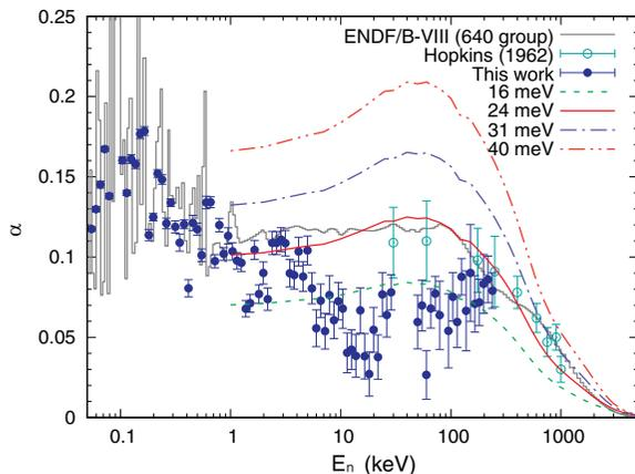
FIG. 18. Statistical model calculations for the neutron-induced reaction on  $^{233}\text{U}$  and comparison of experimental data. The four curves are for different average  $\gamma$ -ray width of 16, 20, 24, and 40 meV.
