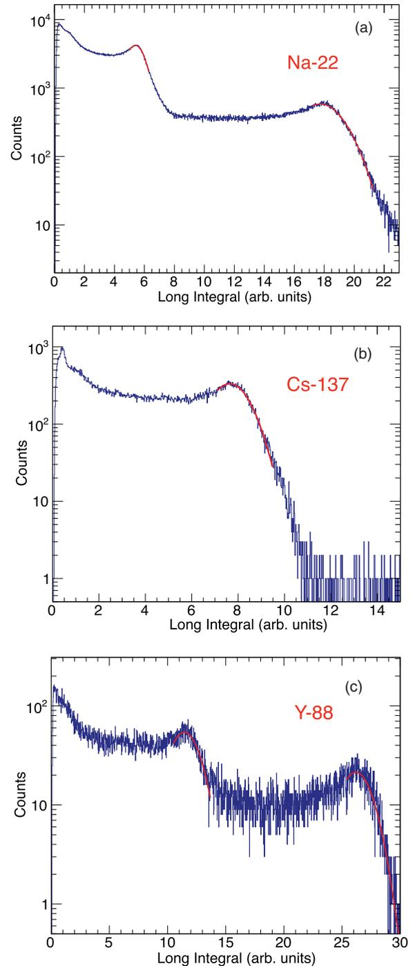
FIG. 6. (a)  $^{22}\text{Na}$   $\gamma$ -ray spectrum with two peaks at 511 keV and 1274.537 keV. (b)  $^{137}\text{Cs}$   $\gamma$ -ray spectrum with a peak at 661.657 keV. (c)  $^{88}\text{Y}$   $\gamma$ -ray spectrum with two peaks at 898.047 keV and 1836.090 keV. All the figures correspond to one of the NEUANCE crystals. The peaks in the spectra have been fitted to Gaussian distribution (in red).
