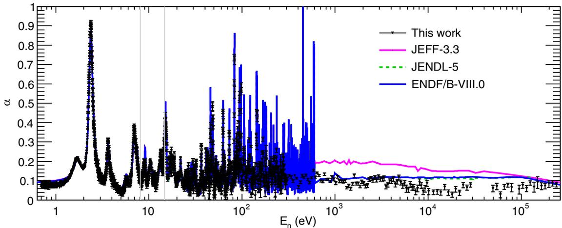
FIG. 9. Capture-to-fission ratio on  $^{233}\text{U}$  (black) compared with ENDF/B-VIII.0 (blue), JEFF-3.3 (magenta), and JENDL-5 (green). The results are shown using 1000 bins/decade from 0.7–100 eV, 500 bins/decade from 100–300 eV, 50 bins/decade from 300–10000 eV, and 25 bins/decade from 100–250 keV. The normalization region is indicated by gray lines. The error bars represent the statistical uncertainties.
