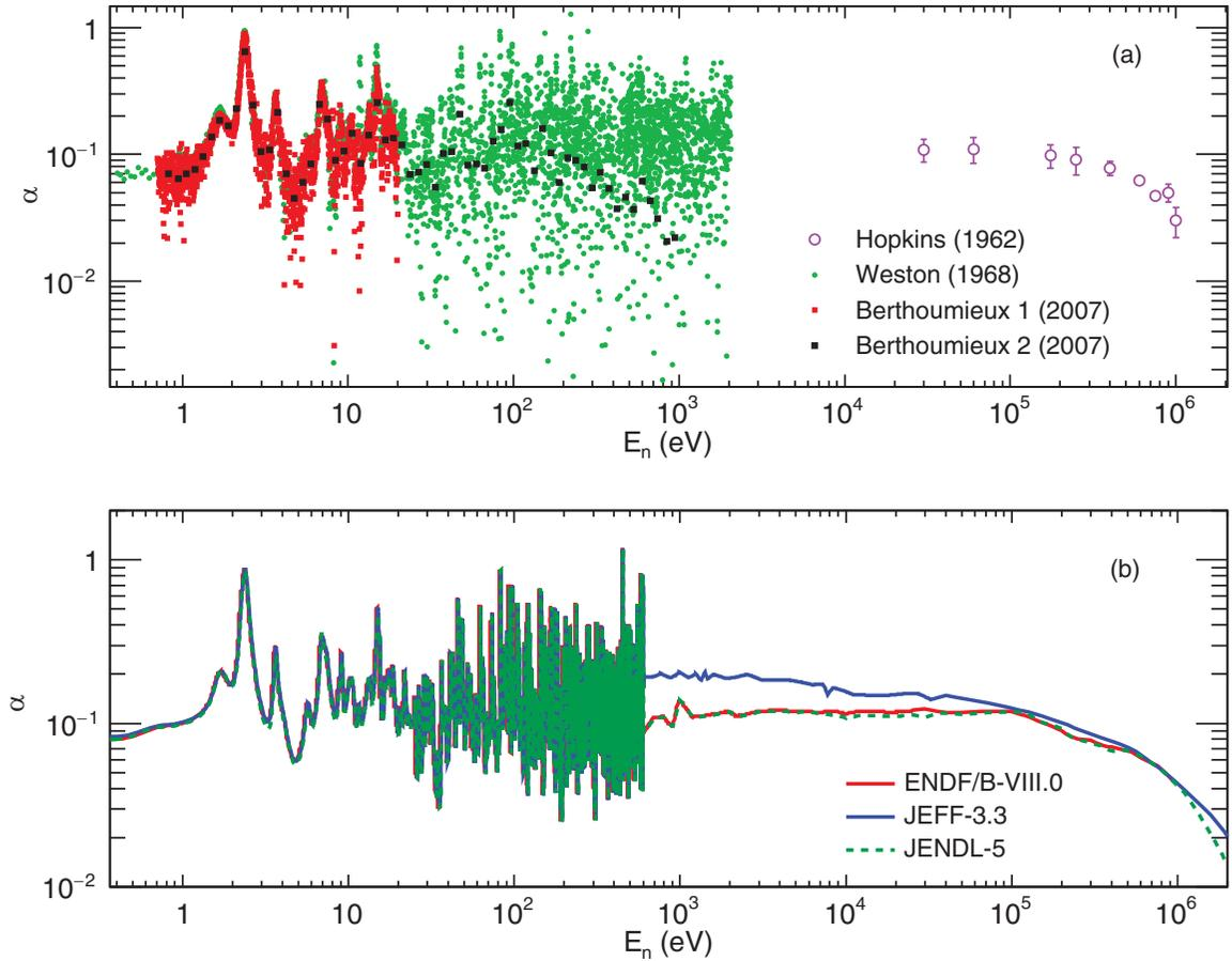
FIG. 1. (a) Existing capture-to-fission ratio data in  $^{233}\text{U}$ , from Weston (1968) [2], Berthoumieux *et al.* (2007) [1], and Hopkins and Diven (1962) [3]. (b) capture-to-fission ratio from ENDF/B-VIII.0, JEFF-3.3, and JENDL-5.
