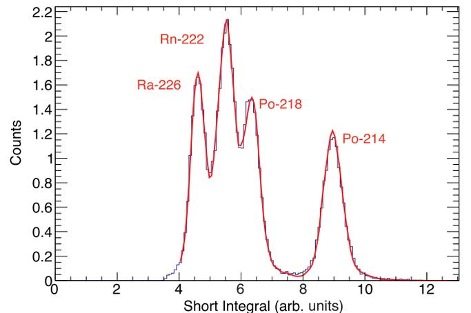
FIG. 4. DANCE  $\alpha$ -particle spectrum for one of the DANCE crystals fitted to a sum of Gaussian distribution (in red) used for the energy calibration. The peaks correspond to the  $\alpha$ -particle decays of  $^{226}\text{Ra}$  (4.8 MeV),  $^{222}\text{Rn}$  (5.5 MeV),  $^{218}\text{Po}$  (6.0 MeV), and  $^{214}\text{Po}$  (7.7 MeV).
