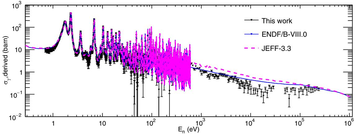
FIG. 17. The  $^{233}\text{U}(n, \gamma)$  cross section calculated multiplying the capture-to-fission cross section ratio by the ENDF/B-VIII.0 fission cross section. The broadened cross section has been used in the resolved resonance region. The results are compared with the ENDF/B-VIII.0 and JEFF-3.3 evaluations. The error bars represent the statistical uncertainties.
