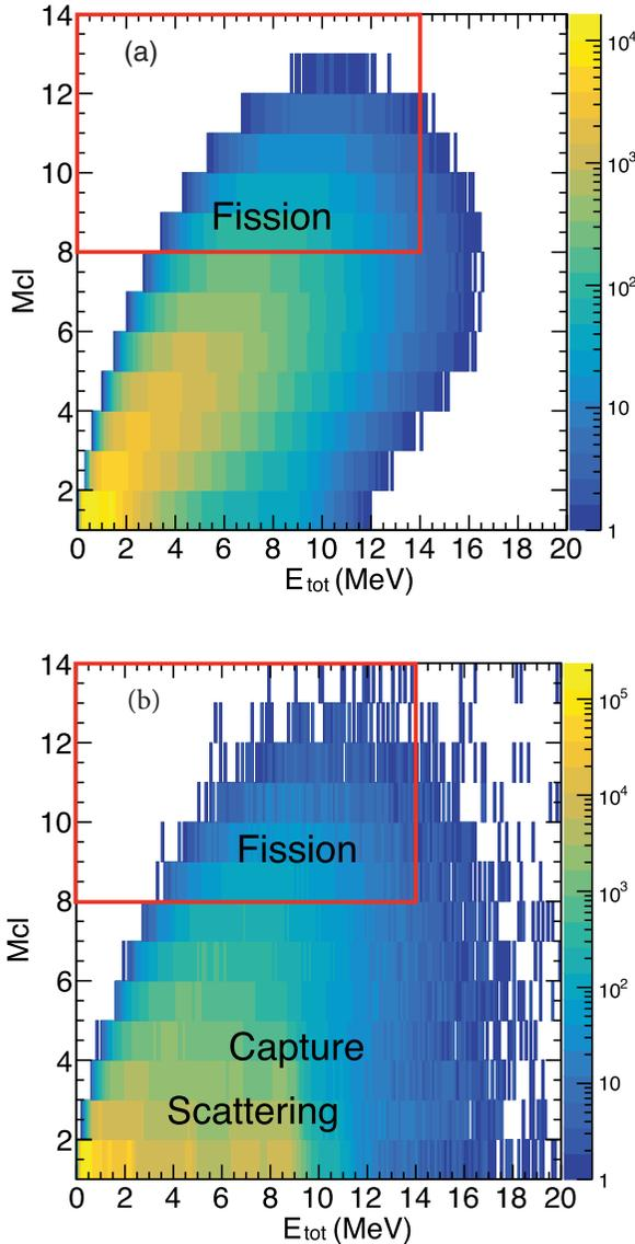
FIG. 7. (a) Cluster multiplicity as a function of the total energy of the  $\gamma$ 's showing the tagged events and (b) the untagged events. The regions where fission, capture and scattering events are dominant are labeled in the figure. The fission normalization window is indicated by the red rectangle.
