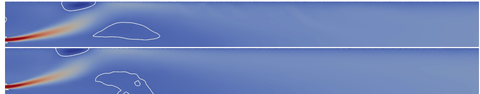
Figure 11. Case A30, grid sensitivity. Longitudinal slice of axial velocity between -30 m/s and 200 m/s. The white iso-contour shows the axial velocity equal to 0. Top: mesh M1, bottom: mesh M2.
