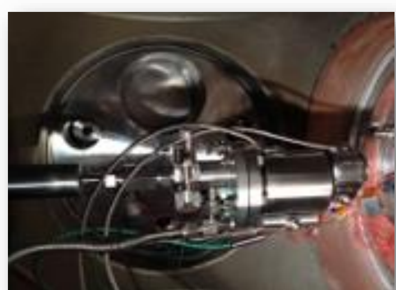
Figure 2b. Home made oven installed in the jet chamber.
