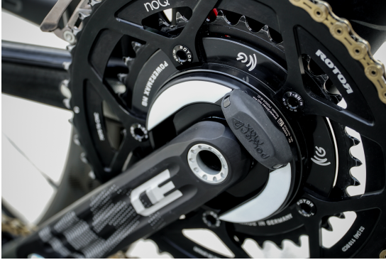
Fig. 1: Picture of a power meter (small grey box) measuring the pedal force. The velocity is measured with a GPS and the power output is calculated as the product of velocity and pedal force.
