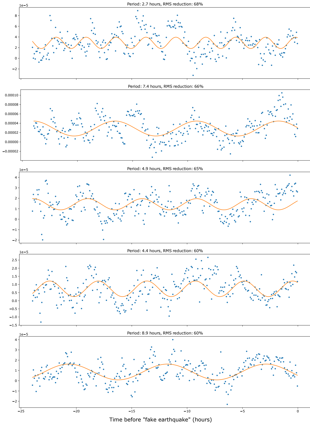
FIGURE S10 – Uniqueness of the sinusoidal signal preceding Tohoku. Sinusoidal fits with misfit reduction above 60% and period below 10 hours obtained over 833 stacks made at random times. None exceeds the 72% of misfit reduction found before the Tohoku earthquake.
