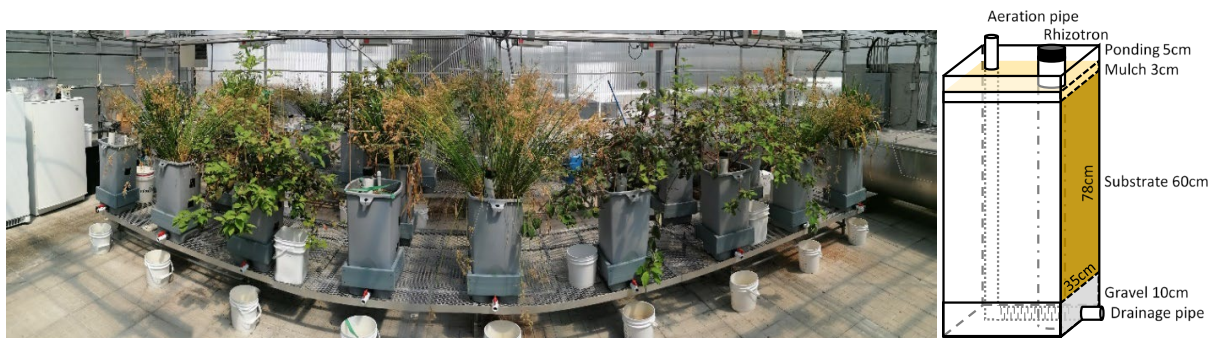
Figure 1. Mesocosm-size bioretention cell experiment (picture July 2020) and mesocosm design.
