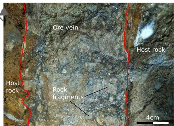
**Figure 5: Picture of the ore vein (delimited by the red lines on the figure) developed in the host rock, filled with galena containing some small host-rock fragments. The ore vein is visible when leaving the fault zone and increases in width.**
