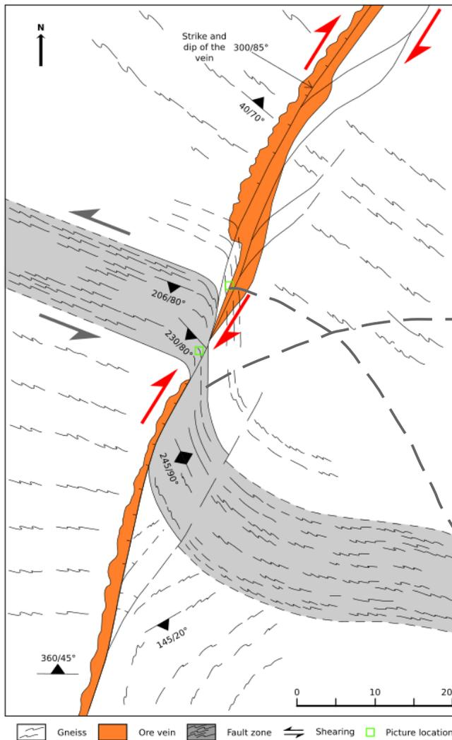
**Figure 3: Geological scheme of the Schauinsland gallery (schematic map view), modified after (Werner et al., 2002). The mine has recorded multiple shearing episodes. The first visible one created the highly sheared zone, called the “Ruschel” in mining language (in grey) with a senestral movement and an E-W direction. The second one crosscuts the Ruschel with a dextral movement and a NNE-SSW direction. The ore vein deposited after the Ruschel shearing. It vanishes close to the**
