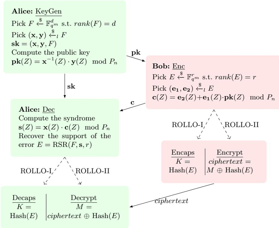
Fig. 1: ROLLO-I (KEM) and ROLLO-II (PKE) cryptosystems.
