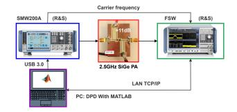
Fig. 10. Synoptic view of the DPD measurement bench.
