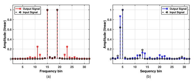
Fig. 3. (a) Normalized Fourier power spectra and (b) normalized Walsh power spectra of a two-tone input (black) and output (red/blue) of a non-linear system.
