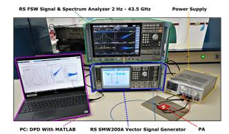
Fig. 11. DPD measurement bench.
