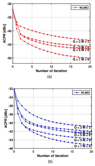
Fig. 16. (a) ACPR evolution over 20 iterations of WLMS for multiple models with a 16-QAM RRC input. (b) ACPR evolution over 20 iterations of WLMS for multiple models with a 64-QAM OFDM input.
