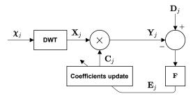
Fig. 5. WLMS block diagram.
