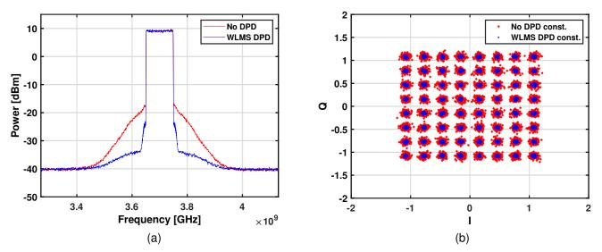
Fig. 15. (a) Power spectrum of PA output with and without DPD after 100 iterations of WLMS algorithm. (b) Output constellation with and without WLMS DPD.
