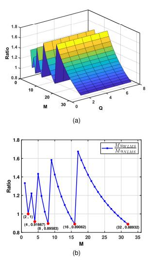
Fig. 8. (a) Ratio of multiplications between WLMS and NLMS for multiple Q and M orders. (b) Ratio of multiplications between WLMS and NLMS for multiple M orders with Q fixed.
