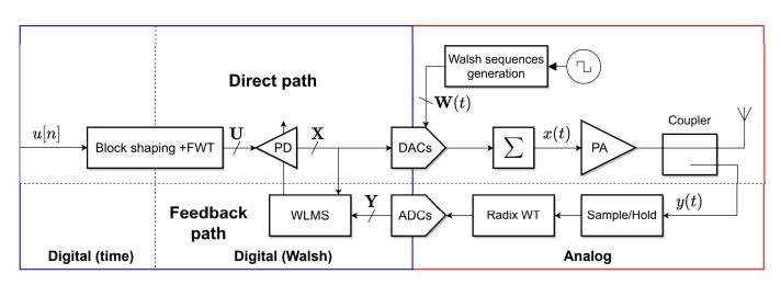
Fig. 14. DPD RF Transmitter based on the WLMS and the Walsh Transform.
