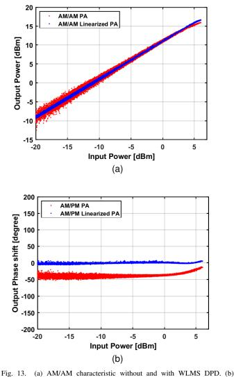
Fig. 13. (a) AM/AM characteristic without and with WLMS DPD. (b) AM/PM characteristic without and with WLMS DPD.
