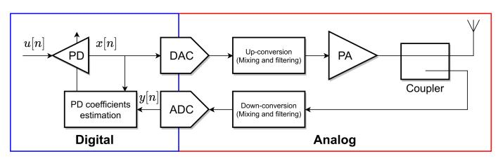
Fig. 1. Typical baseband DPD architecture.
