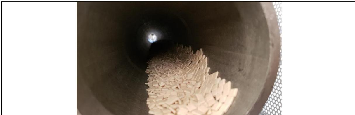
*Figure 1: Crozets moving inside the experimental rotary kiln*
