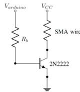
Fig. 9. Electrical circuit for actuating the SMAs.
