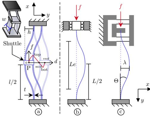
Fig. 4. Representation of a precurved bistable mechanism and the evolution of the force  $f$  as a function of the position  $d$  (subfigure a). The subfigures b and c illustrate respectively a buckling beam with a theoretical guided-fixed end condition and in the real end condition with a slider.
