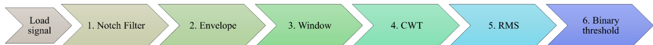
Figure 7: Steps used to process the SR load signal to detect surface damage.
