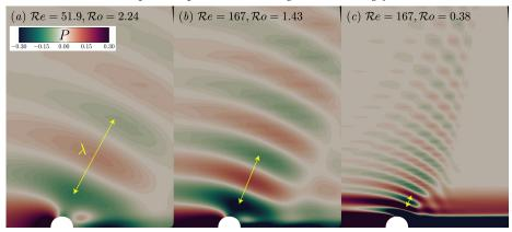
FIGURE 9. Visualization of the inertial wave pattern for several  $\mathcal{R}o$ ; the relative flow with respect to the sphere is from left to right. Colours refer to the amplitude of pressure variations (scaled by  $\frac{1}{2}\rho U_{\infty}^2$ ).
