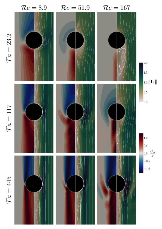
FIGURE 5. Flow structure past the sphere in the parameter space  $(\mathcal{R}e, \mathcal{T}a)$ . The flow is from top to bottom. Left half of the panels (red-blue scale): angular velocity  $U_{\phi}/\sigma$  (scaled by  $U_{\infty}/a$ ); right half (scale of greens): velocity magnitude  $||\mathbf{U}||$  (scaled by  $U_{\infty}$ ) and streamlines in the sphere reference frame.
