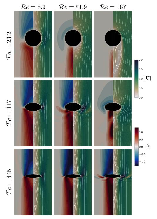
FIGURE 6. Same as figure 5 with the vertical axis compressed by a factor of 2 (resp. 5) for  $\mathcal{T}a=117$  (resp.  $\mathcal{T}a=445$ ) to capture the variations of the vertical extent of the recirculation regions.
