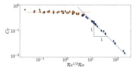
FIGURE 15. Torque coefficient  $C_T$  as a function of  $\mathcal{R}o\mathcal{R}e^{1/2}$ .  $\blacklozenge$  and  $\bigstar$ : results obtained on domains with  $\mathcal{L}=180$  and  $\mathcal{L}\approx 10^3$ , respectively. Blue (resp. orange) colours: configurations corresponding to  $C_D < 6$  (resp.  $C_D \ge 6$ ).
