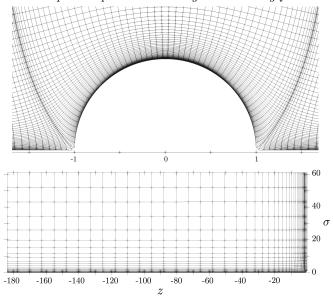
FIGURE 3. Computational grid (pressure nodes stand at the vertices). (a): close-up view in the sphere vicinity; (b)upper semi-domain  $z \leq 0$  with  $\mathcal{L} = 180$  and  $\mathcal{L}_{\sigma} = 60$  (the sphere stands at the bottom right corner; 2 out of 3 cells have been removed in each direction for better visibility).
