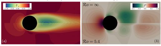
FIGURE 12. Influence of the rigid-body rotation on the velocity and pressure in the sphere vicinity at high Reynolds number ( $\Re e = 300$ ). (a): axial velocity (scaled by  $U_{\infty}$ ); (b): pressure (scaled by  $\frac{1}{2}\rho U_{\infty}^2$ ). Upper half in each frame: non-rotating flow ( $\Re o = \infty$ ); lower half:  $\Re o = 5.4$ . The relative flow with respect to the sphere is from left to right.
