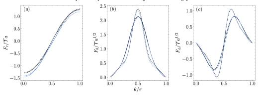
FIGURE 4. Variations of the three components of the surface traction, normalized by  $\rho\nu U_{\infty}/a$ , vs the polar angle  $\theta$ . Blue solid and dashed lines: present results for ( $\mathcal{R}e=5, \mathcal{T}a=55.5$ ) and ( $\mathcal{R}e=2, \mathcal{T}a=445$ ), respectively; black solid and dashed lines: zero- $\mathcal{R}o$  results of Tanzosh & Stone (1994) for  $\mathcal{T}a=50$  and  $\mathcal{T}a=500$ , respectively.
