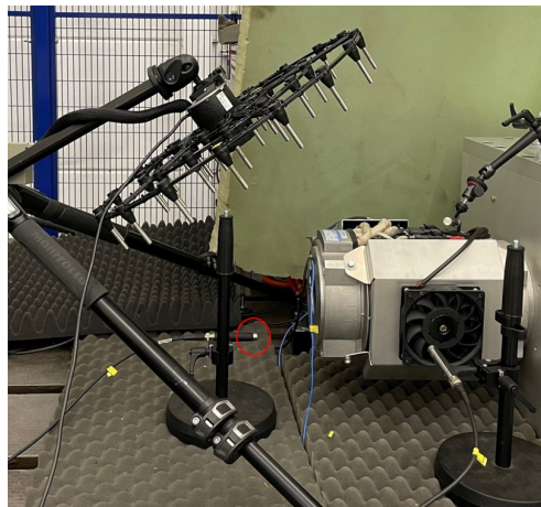
Figure 1: Experimental setup with array facing the induction motor and a reference microphone (marked in red circle).
