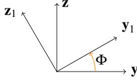
(a) Rotation of the frame  $(x, y, z)$  around  $x$  axis by an angle  $\Phi$
