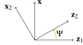
(b) Rotation of the frame  $(x_1, y_1, z_1)$  around  $y_1$  axis by an angle  $\Psi$ . The frame  $(x_2, y_2, z_2)$  is associated with the deformed rotor
