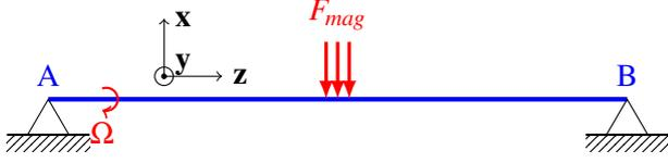
(c) 1D Timoshenko beam of length 50 cm supported at ends A and B, with a constant rotational speed of  $\Omega$ , and magnetic forces applied to the center of the beam over a length of 2 cm.
