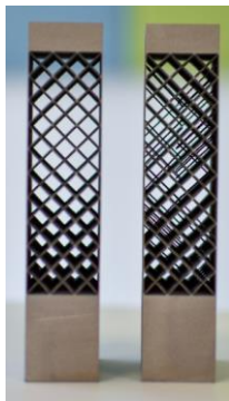
Figure 3 : Manufactured demonstrator (left without resonator ; right with resonators)
