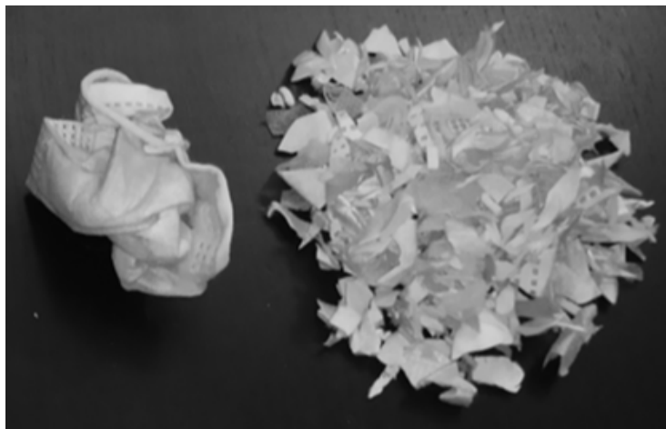
Figure 1: Photograph of crumple and shred specimens (from left to right), each made from one mask.
