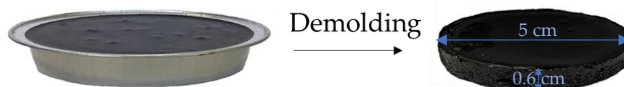
Figure 1. Image of the asphalt cup used for the study before and after unmolding.
