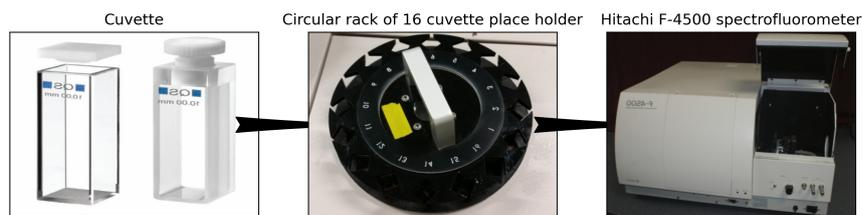
**Figure 3.** Schematic diagram of the experimental setup for EEMs measurements
