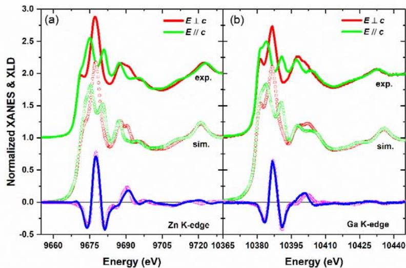
**Figure 2.** Experimental (solid lines) and simulated (open symbols) normalized XANES spectra recorded with two orthogonal linear polarizations and the corresponding XLD spectra for Ga-doped ZnO NWs at the (a) Zn K-edge and (b) Ga K-edge.
