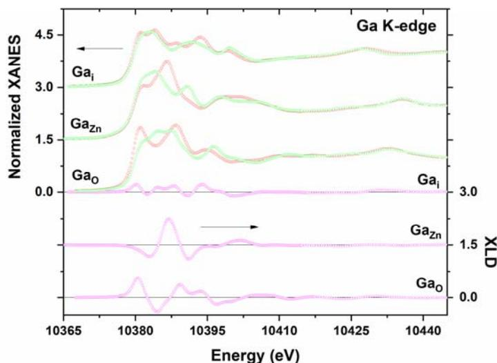
**Figure 3.** Simulated XANES spectra (left scale) for the two orthogonal linear polarizations at the Ga K-edge and the corresponding XLD spectrum (right scale) for three different positions of Ga in the ZnO lattice structure: Ga in a Zn site ( $\text{Ga}_{\text{Zn}}$ ), Ga in an O ( $\text{Ga}_O$ ) site and Ga in an interstitial position ( $\text{Ga}_i$ ). All XANES spectra are normalized to unity and shifted to each other for the sake of clarity.
