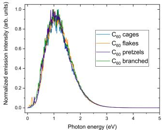
FIG. 4. Emission spectra obtained for  $C_{60}$  carbon clusters at 2400 K in their different structural families.
