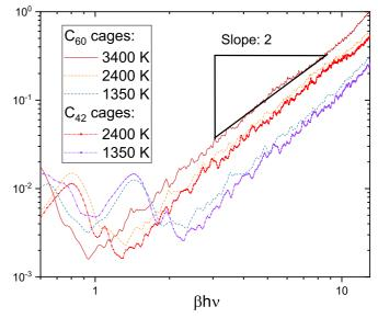
FIG. 6. Mean emissivities for the cage samples of  $C_{60}$  and  $C_{42}$  represented at different temperatures normalized by  $\exp[-(\beta h v)^2/2s]$ , shown as a function of the dimensionless quantity  $\beta h v$ . The quadratic behavior is emphasized in the regime  $\beta h v > 2$ .
