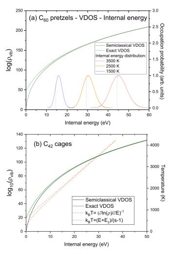
FIG. 9. Vibrational densities of states averaged over the whole sample for (a)  $C_{60}$  pretzels and (b)  $C_{42}$  cages. The relation between internal energy and temperature is obtained by averaging over the whole sample for (a)  $C_{60}$  pretzels. Below 20 eV, the temperatures computed from the exact VDOS and the semiclassical VDOS are significantly different.
