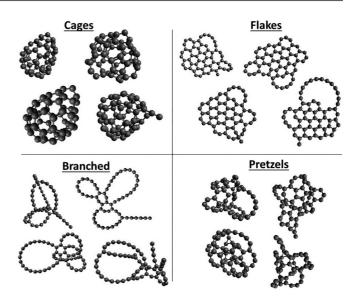
FIG. 1. Typical  $C_{60}$  structures from the four carbon cluster families considered in this work.
