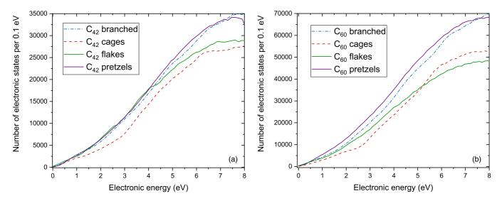
FIG. 5. Electronic densities of states obtained from TD-DFTB data for the four structural families of (a)  $C_{42}$  and (b)  $C_{60}$  cluster samples, accumulated over 1000 isomers in each sample and using a bin size of 0.1 eV.
