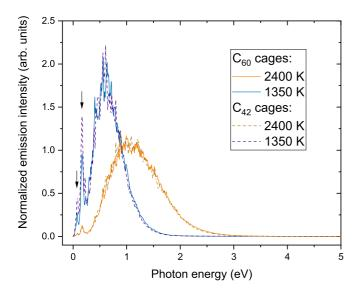
FIG. 3. Emission spectra obtained for  $C_{60}$  and  $C_{42}$  cage samples, at 1350 and 2400 K. The spectra have been convoluted by a Gaussian broadening function with a full width at half maximum of 12.5 meV and they are normalized by their respective integrals. The vertical arrows highlight the positions of vibrational bands.
