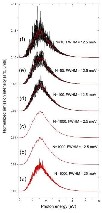
FIG. 8. Emission spectra obtained for  $C_{60}$  cages at 3400 K, using different widths for the Gaussian broadening or different sample sizes: (a)–(c) 1000 isomers with widths of (a) 25, (b) 12.5, and (c) 2.5 meV and (d) 100, (e) 50, and (f) 10 isomers but a constant width of 12.5 meV, the result for the 1000-isomer sample being superimposed as a red curve.
