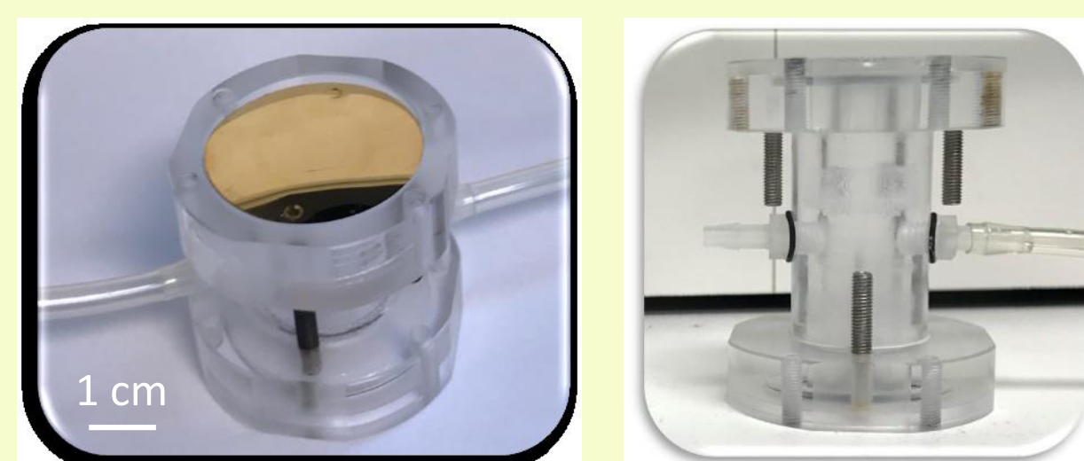
Cell #1: Gold planar electrodes
