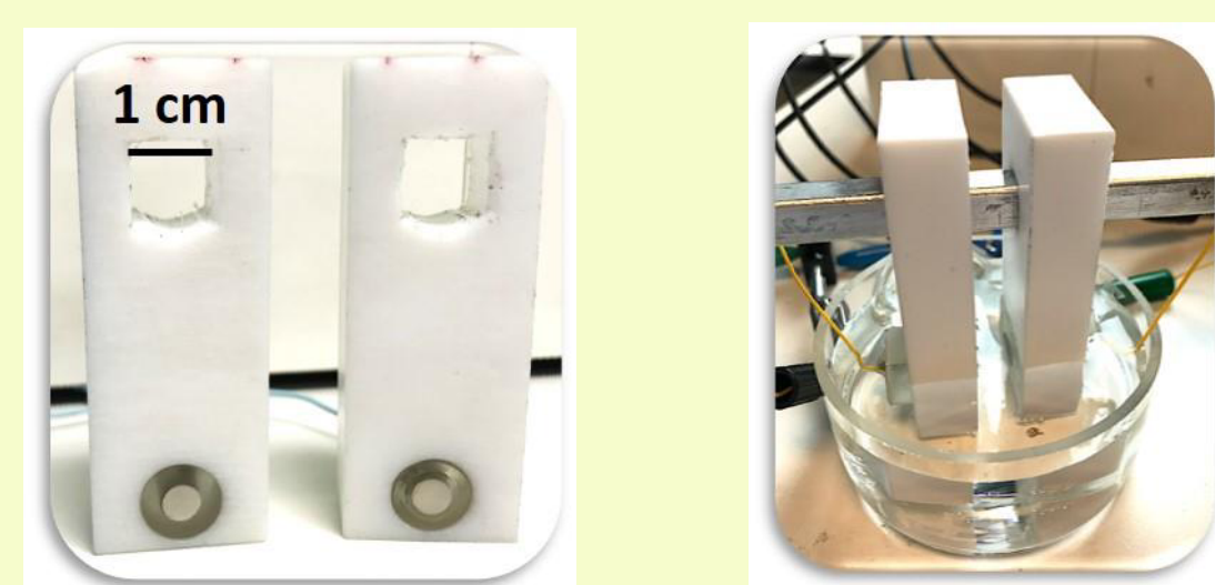
Cell #2: Platinum rod electrodes
