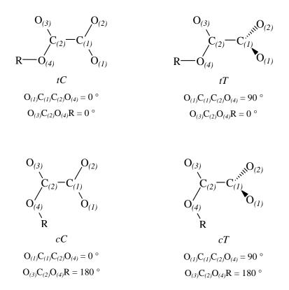
**Scheme 2**: The four conformations of alkyloxalates anions ROCOCOO<sup>-</sup> (R = H, CH<sub>3</sub>, C<sub>2</sub>H<sub>5</sub>, *i*-C<sub>3</sub>H<sub>7</sub>, and *t*-C<sub>4</sub>H<sub>9</sub>) for limiting values of the dihedral angles  $O_{(1)}C_{(1)}C_{(2)}O_{(4)}$  and  $O_{(3)}C_{(2)}O_{(4)}R$ .
