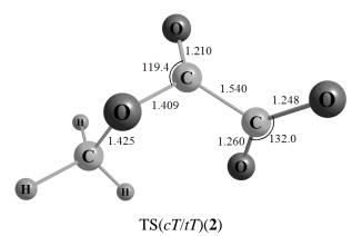
**Figure 3**: Optimized transition structure associated to the passage of the cT to the tT conformation of methyloxalate **2** according to MP2/6-311++G(d) calculations.
