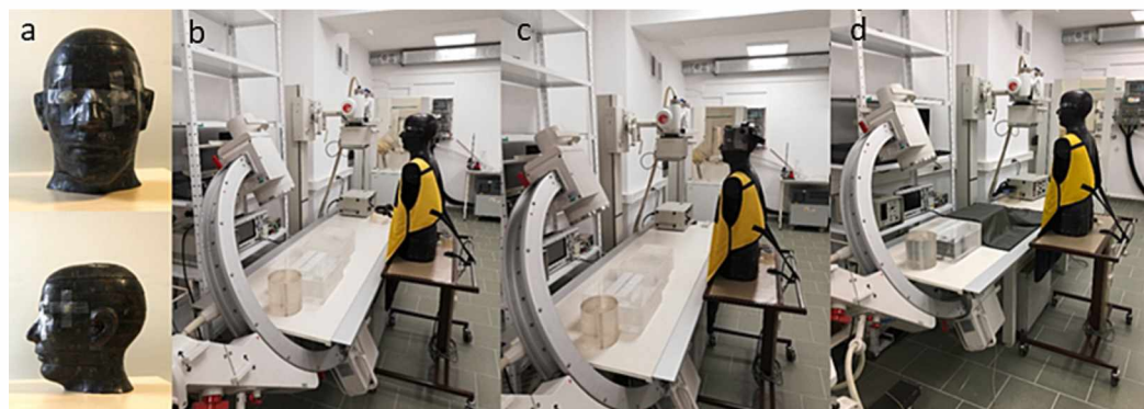
Fig. 6. Measurement of the effectiveness of a mask (model M1) and a lead drape (LITE TECH, Inc., USA) on a RA phantom in a clinical set-up: a: position of dosimeters on the left temple and the eye lens, b: LAO 30 projection with neither mask nor drapes, c: LAO 30 projection with the mask d: LAO 30 projection with the lead drape.
