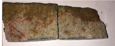
Fig. 11. Penetration depth of chloride ions “X d ” by application of AgNO 3 on cement and GPM with 10% MPCM after 28 days of curing: (A) MCII 0/0/10 ; (B) GPM 100/0/10 ; (C) GPM 90/10/10 ; (D) GPM 80/20/10 .
