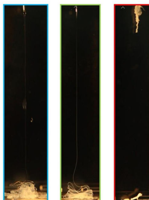
Fig. 3. Wet spinning diagram for (a) N -hexyl- D -galactonamide (GalC6), (b) N -octyl- D -galactonamide (GalC8), (c) N -nonyl- D -galactonamide (GalC9). Blue : gelation in flakes at the bottom of the tank; light green : white gel filament and coil during the fall; dark green : transparent gel filament and coil, which turns white within a few minutes after formation; dark green open square : very thin filament which stacks in thin columns; brown : filament with intermittent clogs; red : clogs at the nozzle exit. Examples of gels obtained in different conditions (with GalC9): photo with blue frame: 20 mg/mL; 100 µL/min; with green frame: 30 mg/mL; 50 µL/min; with red frame: 30 mg/mL; 10 µL/min.
