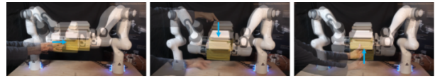
Figure 4. A stack of books is held and moved through physical interaction by a dual-arm robot and a local operator collaborating together.
