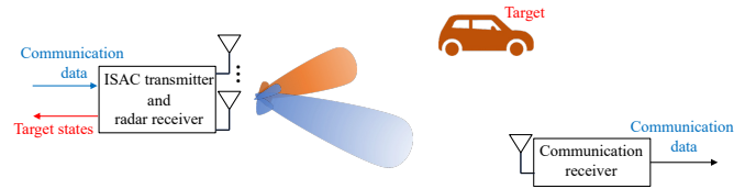
Fig. 1: Considered ISAC scenario with an ISAC transmitter, co-located sensing/radar receiver, and a remote communication receiver. The learned transmit beams provide a flexible trade-off between sensing and communication.
