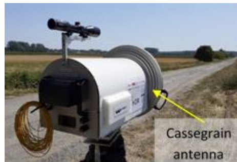
Figure 3: Outdoor validation of the duplexed link over a 645 m distance.
