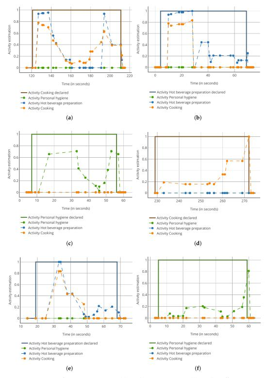
**Figure 5.** Test cases of activity recognition. (a) "Make pasta" test case; (b) "Make coffee" test case; (c) "Go to the toilets" test case; (d) "Prepare a ready-cooked dish" test case; (e) "Make tea" test case; (f) "Have a shower" test case.
