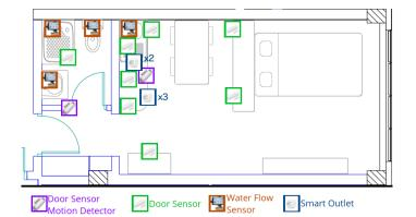
Figure 3. Blueprint of the flat with all the sensor positions.
