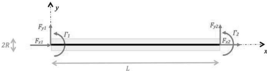
Figure 6. Forces and torques applied on an air-beam.
