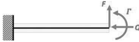
Figure 13. Compressed bended air-beam: notations.
