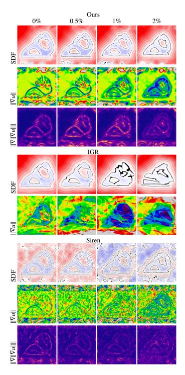
Fig. 13: Slices of the SDF and the gradient's norm of the fertility shape with increasing levels of noise for different INR (variances set to 0, 0.5, 1, and 2% of the shape diagonal). Since IGR's second order derivatives are 0, we do not show  $\|\nabla \| \nabla u \| \|$  for this method.
