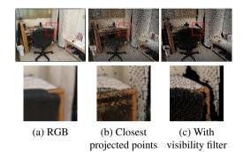
Fig. 3. Visibility filter effect. Points of the table that are occluded by the chair are efficiently discarded. Pixels without geometric information are black.
