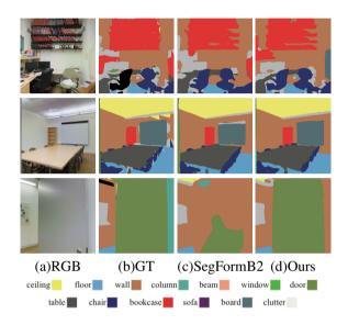
Fig. 7. Segmentation results on the 2D-3D-S validation set using SegFormer-B2 as 2D segmentation network.
