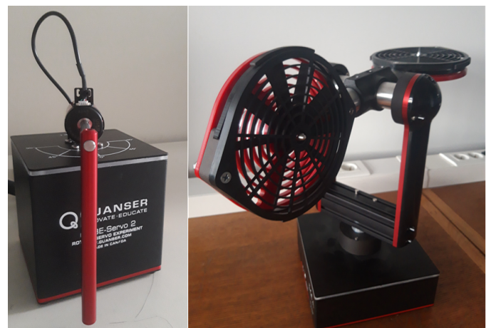
Fig. 2. Example of experimental platforms: Quanser QUBE™-Servo 2 (left) and Quanser Aero 2 (right)
