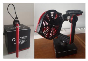
Fig. 2. Example of experimental platforms: Quanser QUBE $^{TM}$ -Servo 2 (left) and Quanser Aero 2 (right)
