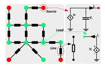
Fig. 1. Meshed DC microgrid network featuring load (•) and source (•) nodes
