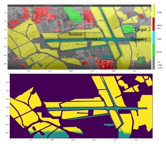
**Fig. 3**. Top: Classification between two target areas (Target 1 and Target 2) of a polarimetric SAR image of Bretigny provided by ONERA using source areas (Source 1 and Source 2). p = 54, n = 2000 (1000 per classes). Bottom: corresponding LS-SVM Classification
