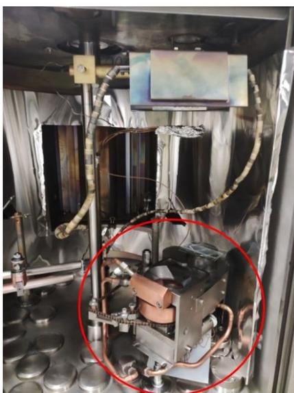
**Fig. 2.** Internal view of the L560 evaporator. The setup is prepared for e-beam evaporation. Inside the red circle one can see the e-beam hearth, the quartz balance and the heating elements. On the bottom left part the electrodes for thermal evaporation are also visible.
