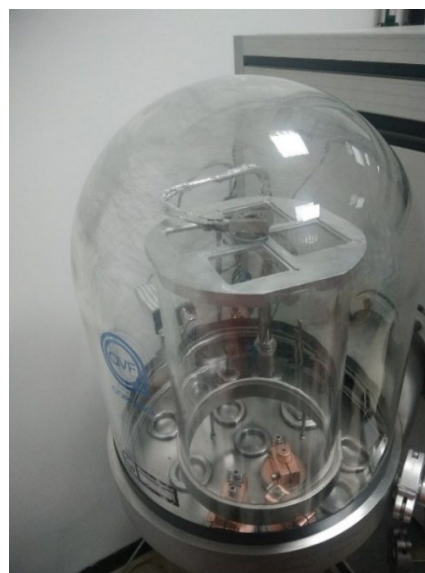
Fig. 1. View of the L300 Thermal Bell Jar evaporator. It is possible to distinguish the glass cylinder on which the target frame holder is placed and the quartz balance at the central upper position.
