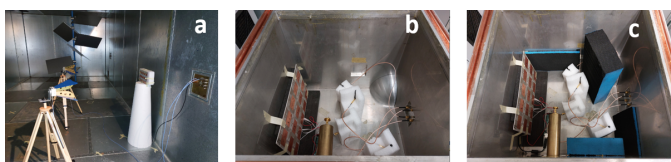
Fig. 5. Photographic images of some experimental setups used to measure the linearity metric under rich-scattering conditions. See Table I for details.
