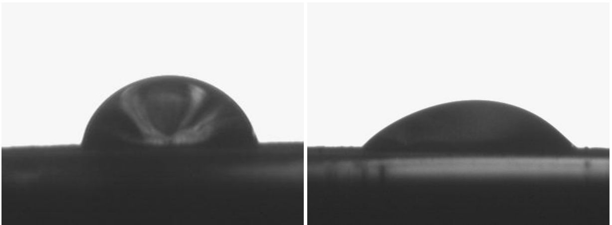
Fig. 2. Two different droplets of deionized water deposited on the PLA scaffold.
