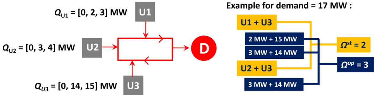
Figure 2. Calculation example of structural and operational multiplicities.
