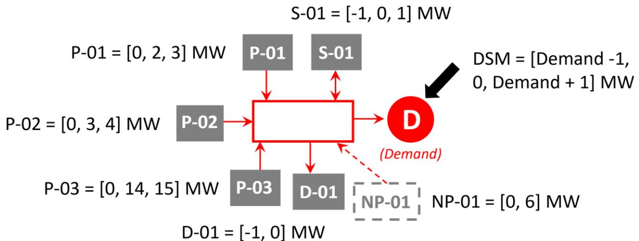
**Figure 3.** Schematical representation of the illustrative case.
