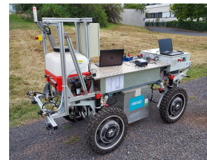
Fig. 8. Experimental robot used for the tests. The collector node is embedded and connected to the CAN bus of the robot.
