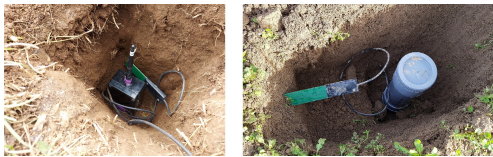
Fig. 1. Sensor nodes with their moisture probe buried at 15 cm deep in a pasture, before being recover by soil
