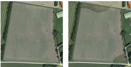
Fig. 12. Trajectories planned in our experimental farm for the mobile robot (interdistance 3.5 m), Google Earth © Digital Globe, 46°20'22.35"N, 3°25'44.28"E. Initial trajectory (left); Modified trajectory due to wetlands assumed to be present in the top left and bottom right corners (right)
